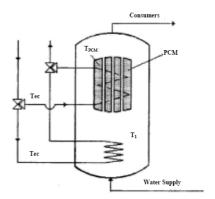
Fig. 5. Scheme of a storage tank (Tec: temperature of energy carrier,  $T_i$ : temperature of the water,  $T_{PCM}$ : temperature of the PCM)
