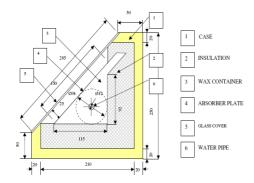
Fig. 9. Schematic of the experimental apparatus cross section
