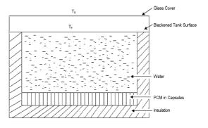
Fig. 1. Solar water heater [25]
