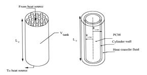
Fig. 2. A cylindrical shell with PCM storage
