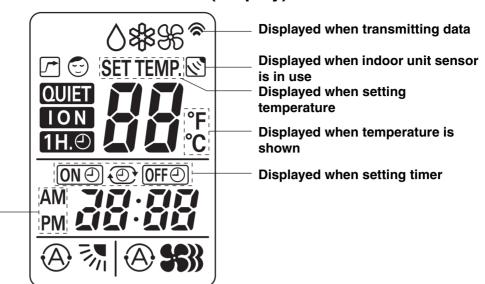
Displayed when the time display is set to 12-hour time.
