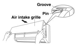
3. Press in the bottom right and left corners of the air intake grille to attach the indoor unit.
