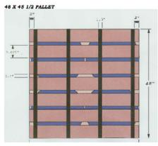
Diagram A: Pallet design 1 for UN1H1 and UN1H2 plastic drums.
