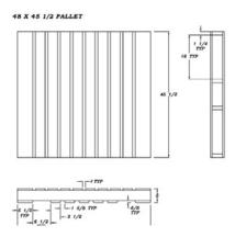
Diagram C: Pallet design 3 for UN1H1 and UN1H2 plastic drums.
