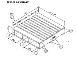
Diagram B: Pallet design 2 for UN1H1 and UN1H2 plastic drums.
