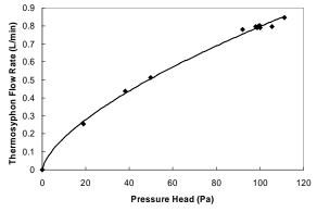
Fig. 5. Plot of experimental results showing the dependence of the thermosyphon flow rate on the pressure head (Cruickshank et al, 2006c).
