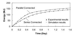
Fig. 11. Total energy delivered to the storage.
