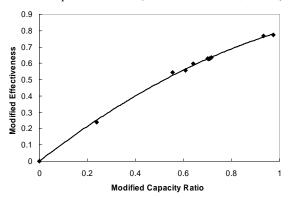
Fig. 6. Experimentally derived modified effectiveness as a function of modified capacity ratio (Cruickshank et al, 2006c).
