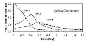
Fig. 8. Individual charge rates across each heat exchanger for the series configuration.
