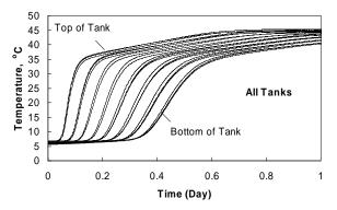
Fig. 9. Measured temperature profile of the parallel connected storage tanks during charging.
