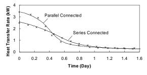
Fig. 10. Charge rate across all heat exchangers.
