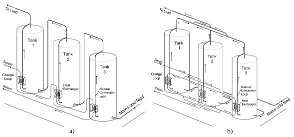
*Fig. 1. Multi-tank storage configurations studied: a) series-connected for charge and discharge, and b) parallel-connected for charge and discharge.*
