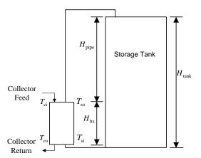
Fig. 4. Illustration of a NCHE heat exchanger showing location of reference temperatures.
