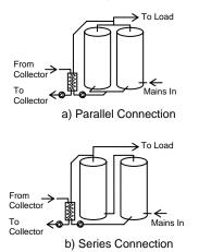
Fig. 3. Parallel and series connected hot water storage tanks charged through a collectorside heat exchanger.
