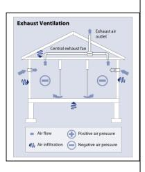
Spot ventilation exhaust fans installed in the bathroom properly designed and installed to operate continuously represent an exhaust ventilation system in its simplest form.
