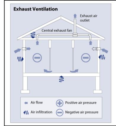
Spot ventilation exhaust fans installed in the bathroom properly designed and installed to operate continuously represent an exhaust ventilation system in its simplest form.
