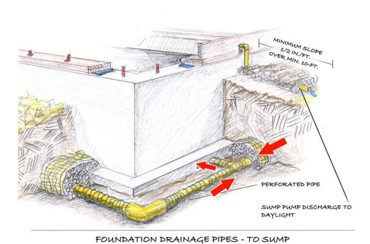
**Figure 5** - Properly Installed Drain Tile Discharging to a Sump Pit. This image shows the exterior of the foundation and placement of the drainage tile that diverts water to the sump pit.
