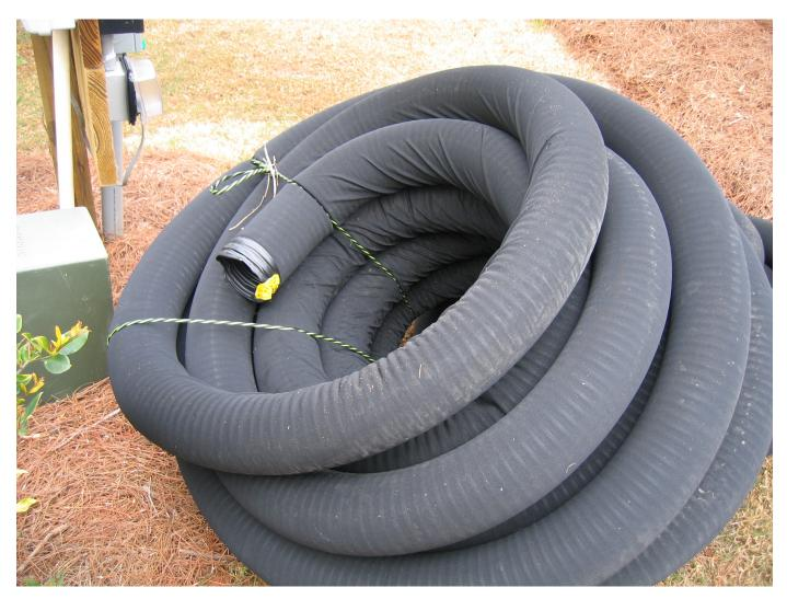
**Figure 1** - Drain Tile with Protective Cover. Drain tile is not tile at all but actually corrugated pipe with small perforations. This image shows drain tile with a protective filter cover that keeps silt and sand from clogging the system.
