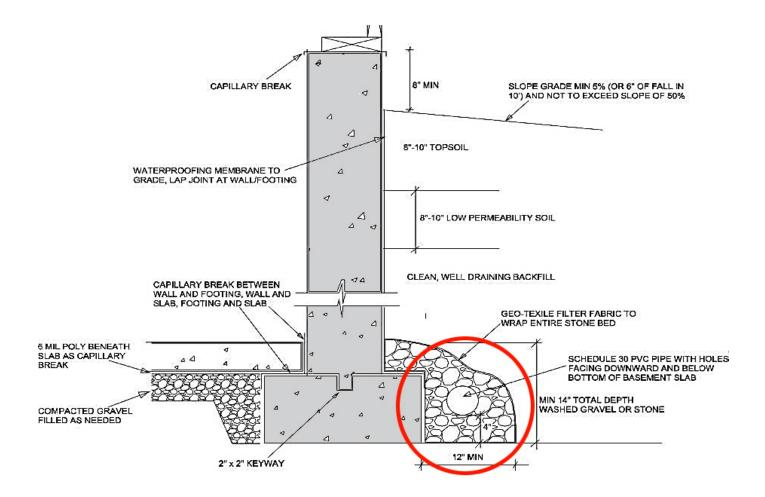
**Figure 2** - Drain Tile Cross-Section. This image shows the relative placement of the drain tile to the foundation wall. Note that the geo-textile filter fabric must be installed to cover the entire bed of gravel in the trench.
