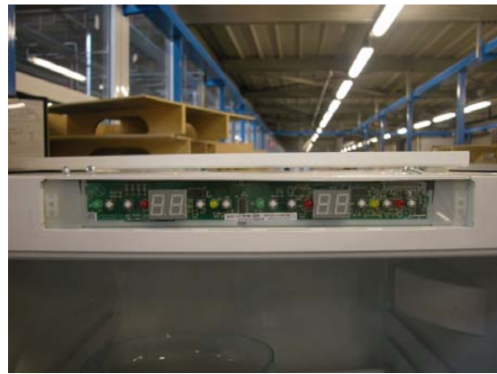
c) Remove the programme plate removing the 2 screw covers and the 2 fixing screws.
