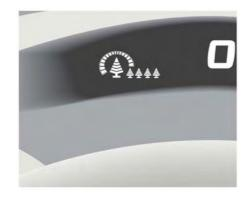
While the vehicle is being driven you can check your own ECO drive level on the ECO indicator. See "ECO indicator" in the "2. Instruments and controls" section.
