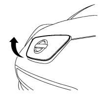
Put your hand into the under side of the lid and open until it is in the fully open position.
