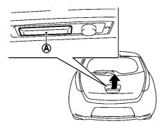
To open the rear hatch, unlock it and push the rear hatch opener switch (A). Pull up the rear hatch to open.
