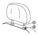
To lower, push and hold the lock knob and push the headrest down.
