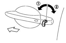
You can switch the lock system to the mode that allows you to open all the doors when the key is turned once. (See the LEAF Navigation System Owner's Manual.)
