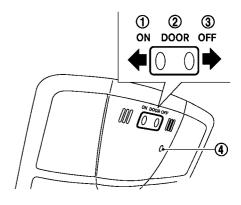
The map light control switch has three positions: ON 1, DOOR 2 and OFF 3.
