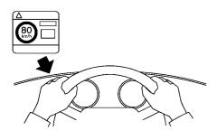
Open the lid of the air compressor and take out the speed restriction sticker, then put it in a location where the driver can see it while driving.
