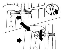
If the electric parking brake cannot be released by operating the electric parking brake switch, the parking brake can be mechanically released.
