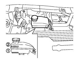
Check the fluid level in the reservoir. If the fluid is below the MIN line (1) or the brake warning light illuminates, add Genuine NISSAN Super Heavy Duty Brake Fluid or equivalent DOT 3 fluid up to the MAX line (2). If fluid must be added frequently, the system should be checked by a NISSAN certified LEAF dealer.
