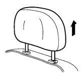
The illustration shows the seating positions equipped with adjustable headrests.
