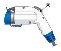
When recharging outside such as in your drive way, use a commercially available padlock attached in position (A) to prevent theft.
