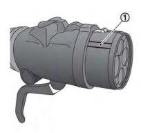
4. Align ① with the groove of the charge port and insert the charge connector.
