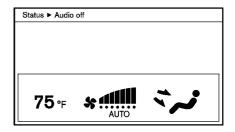
Push the STATUS button to display the climate control system status on the navigation system screen. (See the LEAF Navigation System Owner's Manual.)
