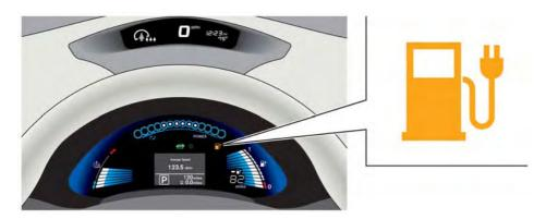
If the low battery charge warning light illuminates, the Li-ion battery charge is too low for travel. See "Low battery charge warning light" in the "2. Instruments and controls" section. Charge the Li-ion battery as soon as possible.
