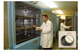
Constant temperature and humidity chambers – water vapour diffusion
