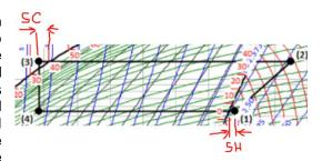
suction inlet of the compressor (after the cap tube has warmed it slightly), and using the appropriate gas chart - there's even an iphone app for it! It's hard to measure the temperature accurately – the best I found was a thermocouple cable taped to the pipe firmly by the suction inlet, then insulated.
