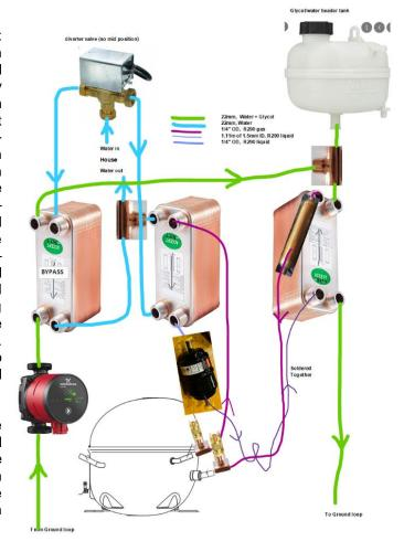
The compressor circuit was mounted to a portable structure, and the ground loop pump etc in a more fixed way. The heatpump water connections are made with rubber washer compression fittings, for ease of removing the central heatpump for any maintenance in future.
