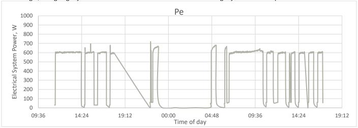
For the below DHW heating graph the bathroom radiator is off, DHW is now permitted to run to 45C, and is showing recovery after a long shower. The COP (graph shows scaled elec and thermal power, see legend) seems oddly stable and at 4 between 25C and 45C output, I had expected it to fall – maybe measurement inaccuracy?
