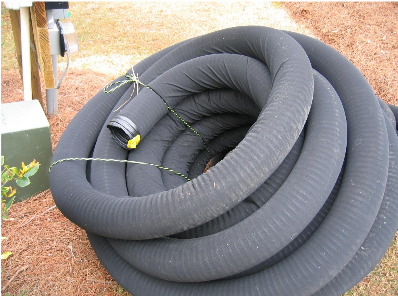
**Figure 1** - Drain Tile with Protective Cover. Drain tile is not tile at all but actually corrugated pipe with small perforations. This image shows drain tile with a protective filter cover that keeps silt and sand from clogging the system.
