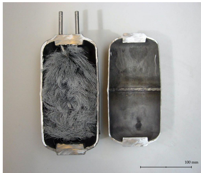
Figure 2. Cut tank brush heat exchanger.
