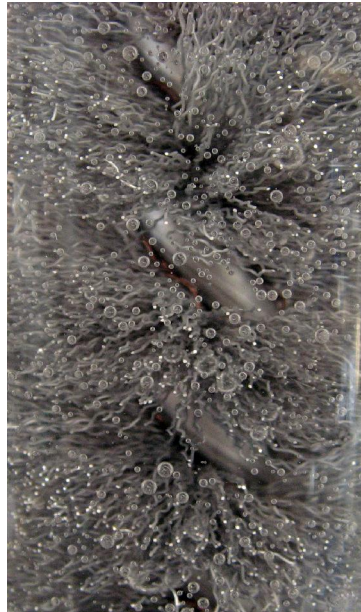
Figure 42. Gas bubbles in liquid sodium acetate trihydrate and water mixture melted with brush heat exchanger.
