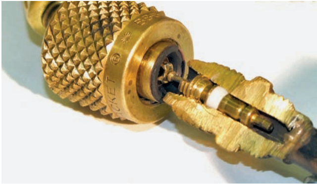
Figure 25-15 The core depressor on the refrigerant hose pushes in the Schrader valve core when the hose is connected
