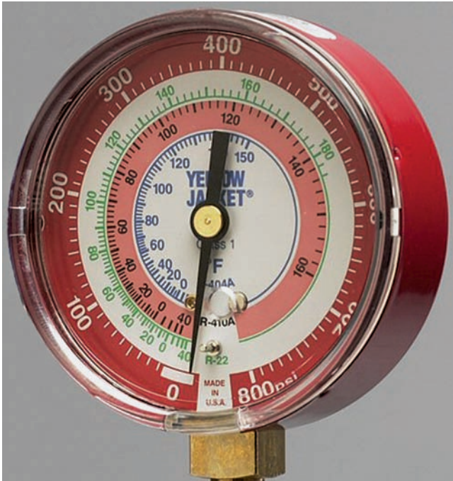
Figure 25-25 High side pressure gauge for R-410a (Courtesy of Ritchie Engineering Company, Inc.—Yellow Jacket® Products)
