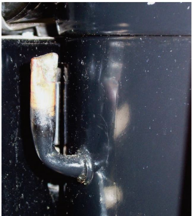
Figure 25-40 Process tube on hermetic compressor
