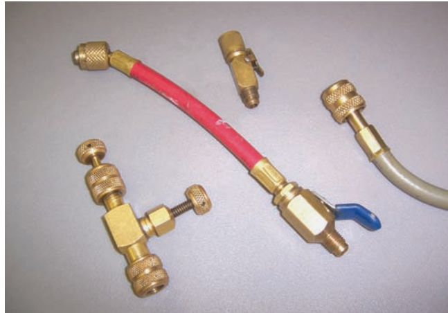
Figure 25-36 Positive shut-off adapters make connecting to Schrader valves easier
