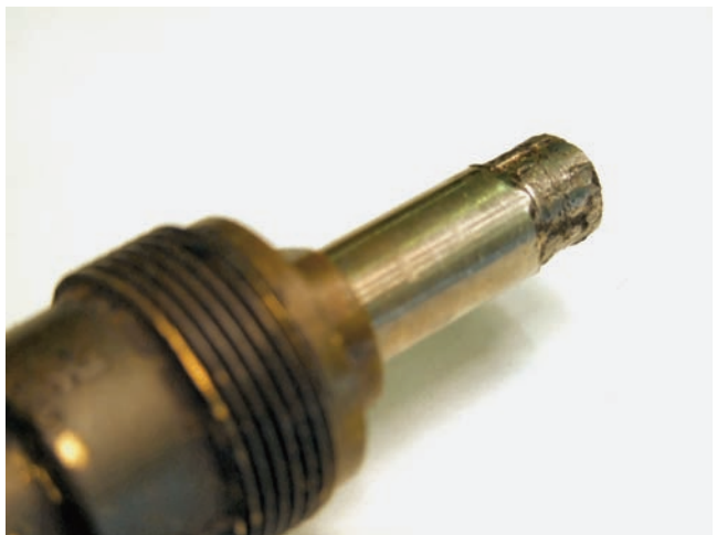
Figure 25-13 This valve stem has been ruined by a careless technician using the wrong tool
