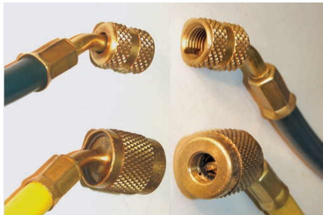
Figure 25-37 The hoses at the top of the picture have a standard Schrader core depressors. The hoses on the bottom of the picture have automatic check valves built in that keep the refrigerant in the hose from coming back out when the hose is removed.
