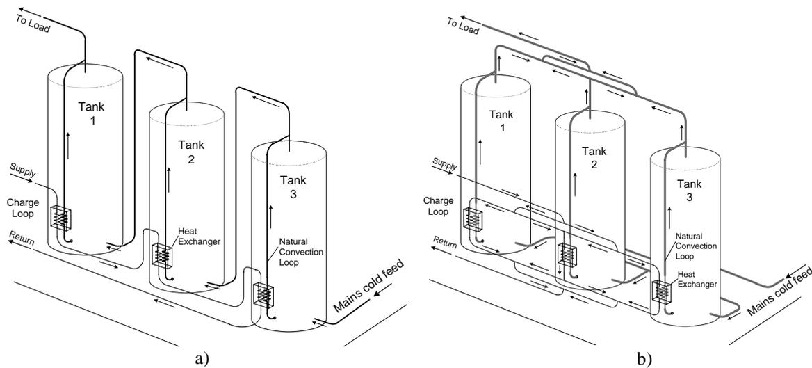
Fig. 1. Multi-tank storage configurations studied: a) series-connected for charge and discharge, and b) parallel-connected for charge and discharge.
