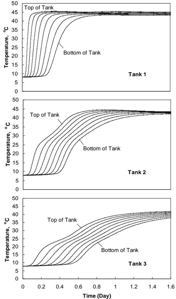
Fig. 7. Measured temperature profile of the series connected storage tanks during charging.
