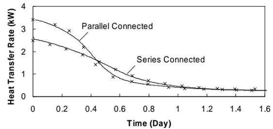
Fig. 10. Charge rate across all heat exchangers.
