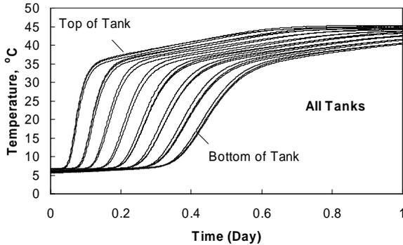
Fig. 9. Measured temperature profile of the parallel connected storage tanks during charging.
