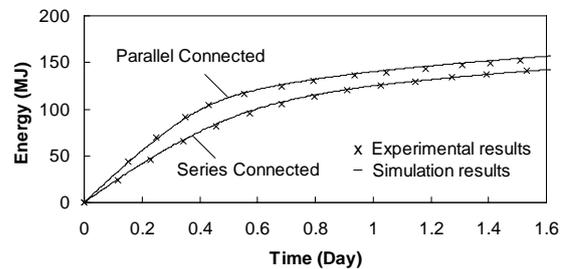
Fig. 11. Total energy delivered to the storage.
