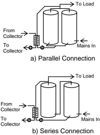
Fig. 3. Parallel and series connected hot water storage tanks charged through a collector-side heat exchanger.
