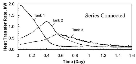
Fig. 8. Individual charge rates across each heat exchanger for the series configuration.
